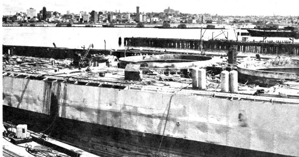
By June, 1960, the battleship Colorado had been cut down to the point where no part of the ship intruded into the view of Seattle's skyline as seen from the work pier. The four vertical tanks seen on the deck at the right contained propane gas for the cutting torches. About this time, natural gas was piped to the shipyard and was used to cut up the rest of the big vessel.
